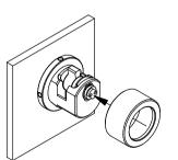
5 Mount cam in accordance with the assembly instructions of article no. 7480, 7481 or 7482
