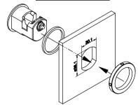
For material thickness of 7 and 4mm a total of 2 or 3 space washers (article no. 2618) are needed, available separately.
